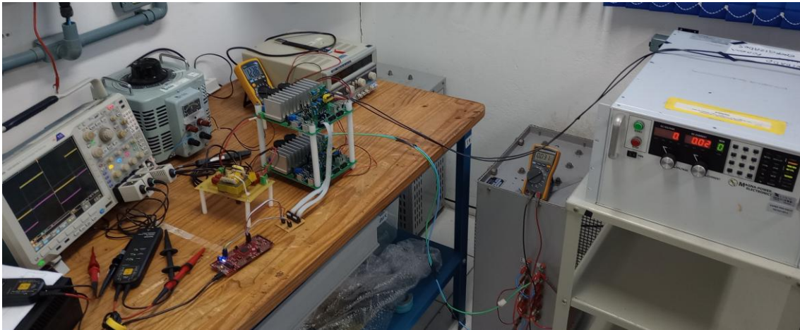
Figure 42 – Setup for experimental tests with prototype for SPS modulation.
