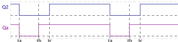
Fig. 5 Switches commands in "step down" mode
