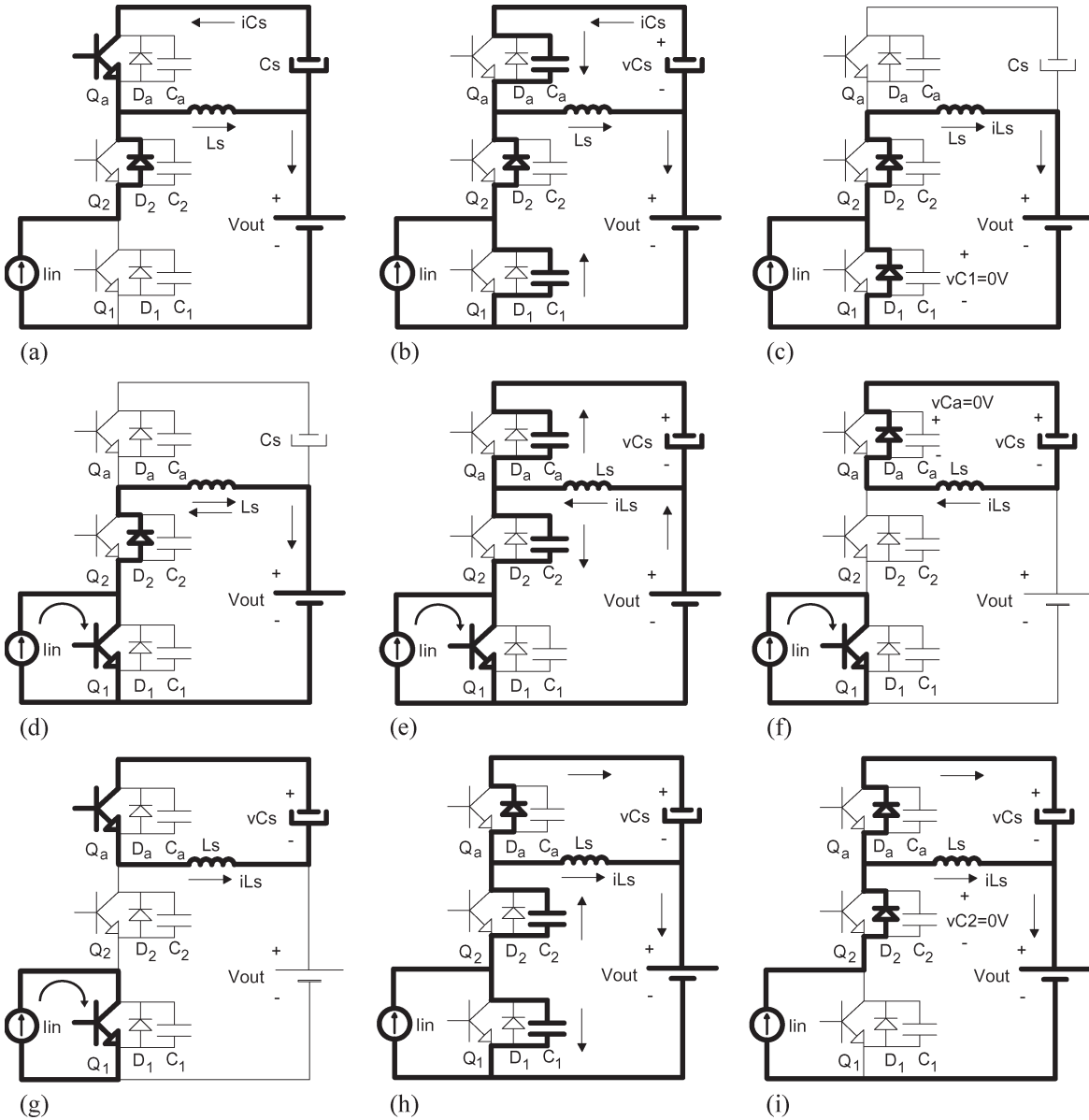
Fig. 4. Operation stages. (a) First stage ( t_0-t_1 ). (b) Second stage ( t_1-t_2 ). (c) Third stage ( t_2-t_3 ). (d) Fourth stage ( t_3-t_4 ). (e) Fifth stage ( t_4-t_5 ). (f) Sixth stage ( t_5-t_6 ). (g) Seventh stage ( t_6-t_7 ). (h) Eighth stage ( t_7-t_8 ). (i) Ninth stage ( t_8-T_s+t_0 ).
