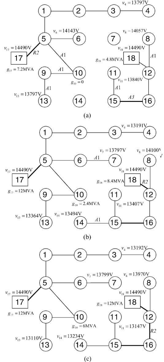
Fig. 4. Solution for multistage expansion with distributed generation:  $C = 1040.82$ . (a) Stage 1:  $c_1^{inv} = 686.00$  e  $c_1^{oper} = 14.00$ . (b) Stage 2:  $c_2^{inv} = 241.00$  e  $c_2^{oper} = 26.00$ . (c) Stage 3:  $c_3^{inv} = 40.00$  e  $c_3^{oper} = 41.20$ .
