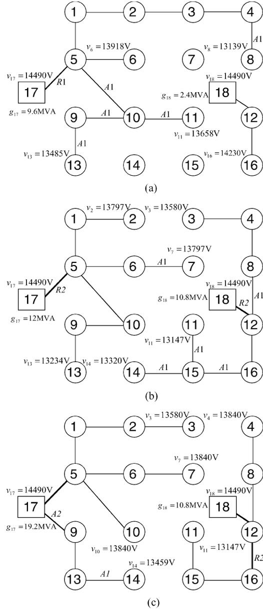
Fig. 2. Solution with year-by-year expansion:  $C = 1488.79$ . (a) Stage 1:  $c_1^{\text{inv}} = 506.00$  and  $c_1^{\text{oper}} = 13.00$ . (b) Stage 2:  $c_2^{\text{inv}} = 593.00$  and  $c_2^{\text{oper}} = 16.00$ . (c) Stage 3:  $c_3^{\text{inv}} = 473.00$  and  $c_3^{\text{oper}} = 16.00$ .
