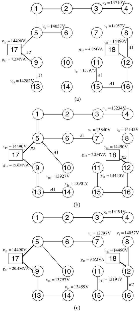
Fig. 3. Solution with multistage expansion:  $C = 1162.48$ . (a) Stage 1:  $c_1^{inv} = 743.00$  e  $c_1^{oper} = 13.00$ . (b) Stage 2:  $c_2^{inv} = 367.00$  e  $c_2^{oper} = 16.00$ . (c) Stage 3:  $c_3^{inv} = 40.00$  e  $c_3^{oper} = 16.00$ .
