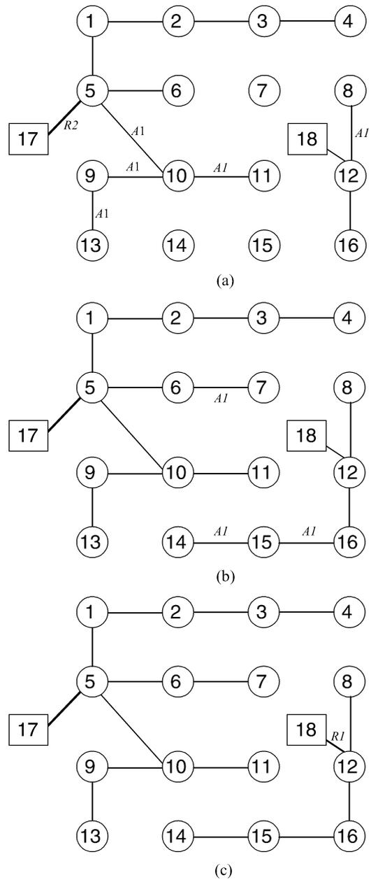
Fig. 6. Solution for multistage expansion with distributed generation considering three load levels:  $C = 940.76$ . (a) Stage 1:  $c_1^{\text{inv}} = 532.00$  and  $c_1^{\text{oper}} = 13.00$ . (b) Stage 2:  $c_2^{\text{inv}} = 316.00$  and  $c_2^{\text{oper}} = 22.46$ . (c) Stage 3:  $c_3^{\text{inv}} = 19.00$  and  $c_3^{\text{oper}} = 45.37$ .
