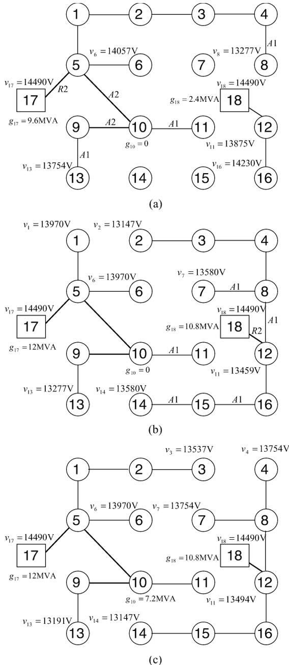
Fig. 5. Solution for multistage expansion with distributed generation and constrained investment:  $C = 1075.91$ . (a) Stage 1:  $c_1^{\text{inv}} = 564.00$  and  $c_1^{\text{oper}} = 13.00$ . (b) Stage 2:  $c_2^{\text{inv}} = 453.00$  and  $c_2^{\text{oper}} = 16.00$ . (c) Stage 3:  $c_3^{\text{inv}} = 0.00$  and  $c_3^{\text{oper}} = 46.00$ .
